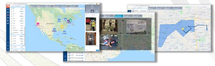
Dispatch applications can track multiple user locations and travel routes with job site time stamps to manage and dispatch remote workers. Dispatchers can draw geofences on the map to define boundaries for territories and service areas. Alarms can be generated when users enter or leave a geofenced areas. Note that location tracking is GPS based, which does not track locations of indoor users in a large facility like a convention center.
