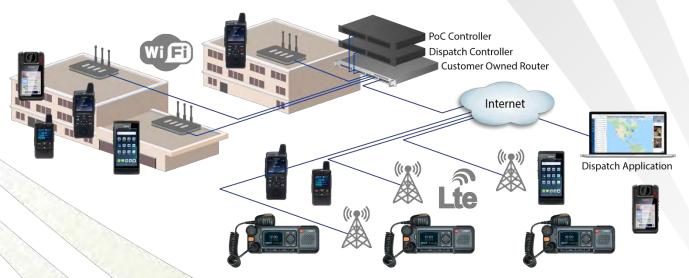
The PoC devices on the nationwide 4G/LTE network use SIM cards to access the mobile operator's cellular network with an Access Point Name (APN) that routes the data traffic to the mobile operator's internet gateway. The PoC controller accesses the internet through the customer's network router.
